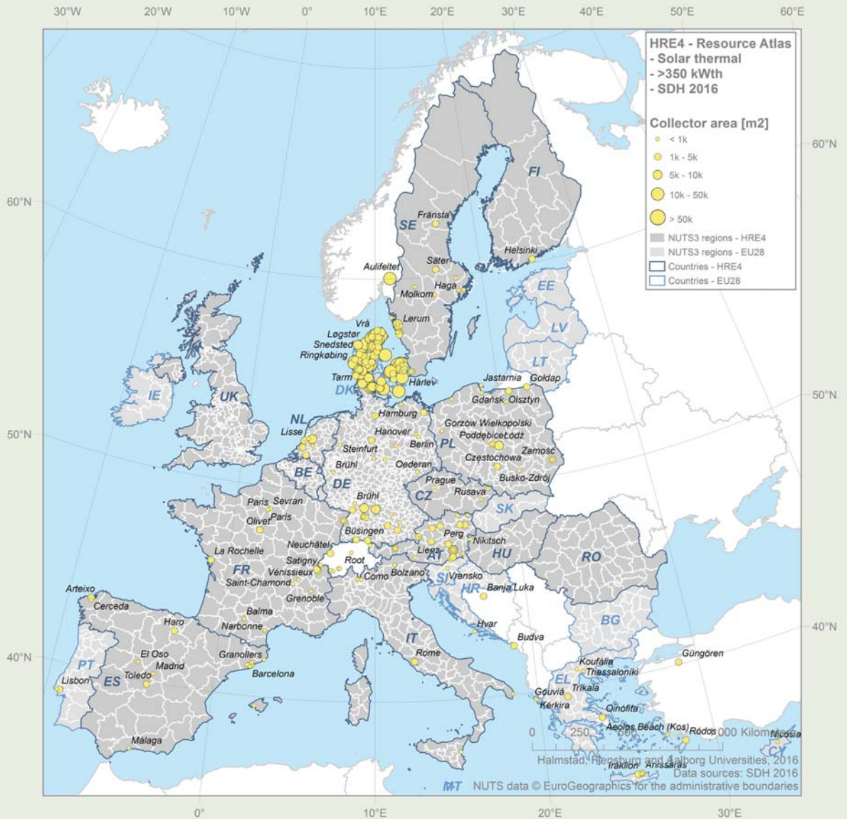
Figure 7: Solar district heating systems >500 m 2 (350 kWh th ) in Europe. (Source: Heat Roadmap Europe)
